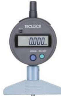
DMD-2130S2 φ3.2mm강구 측정자타입 최소표시량0.001mm 측정범위12mm
